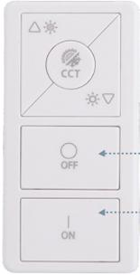
Long press the ON and OFF button simultaneously for 10 seconds to activate commissioning mode
